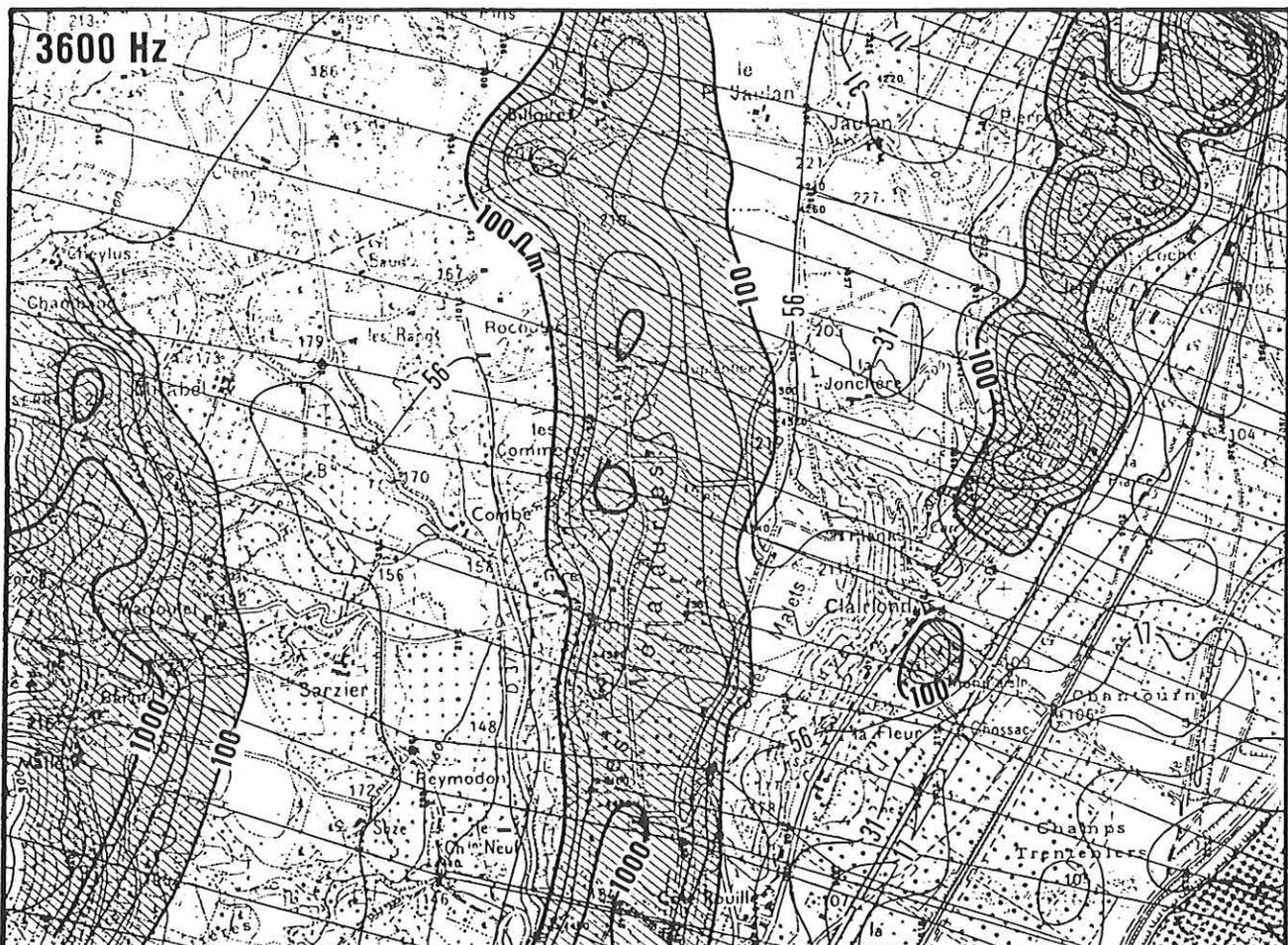
**Fig.6** ELECTROMAGNETISME HELIPORTE, RECHERCHE DE FAILLE EN TERRAIN GRANITIQUE
