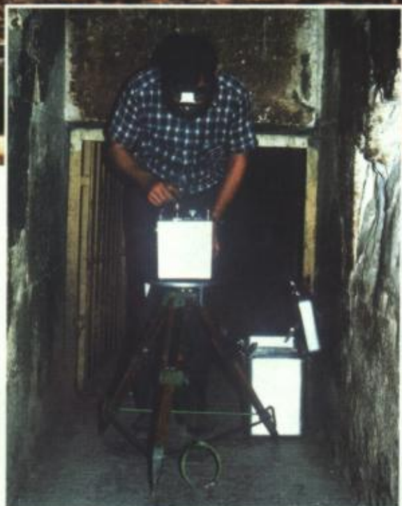
Vertical gravity gradient measurement (1 m off the ground!)
